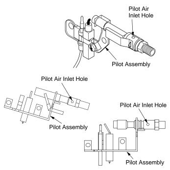
Figure 39 - Pilot Inlet Air Hole (Your pilot may vary from pilots shown)
